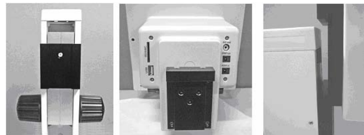
The dove-tail groove on trestle
