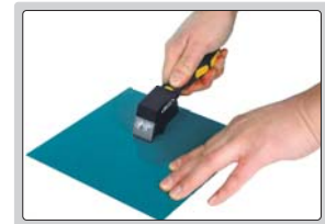
step 1: make grid cutting on surface
