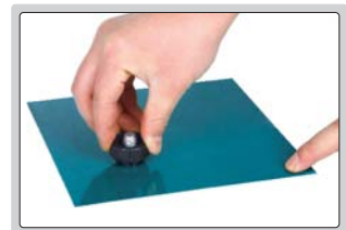
step 2: cut the paint around dolly by using ring cutter
