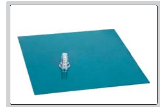
step 1: glue the dolly on the paint coating
