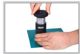
step 3: rotate the handwheel, read the adhesion when dolly is pulled off
