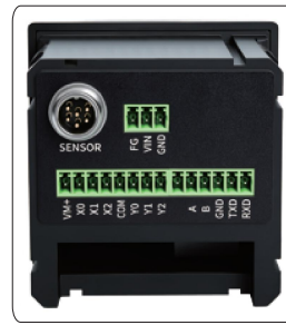
IO output and communication ports (included) type B (back view)
