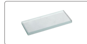
50mm reading scale (check magnification accuracy)
