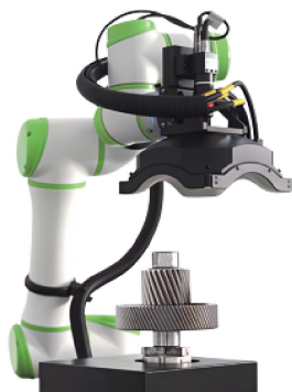
coordinating with a robot arm to capture real-time images and detect defects on rotating gears
