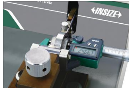
lapping measuring surfaces of outside micrometer
