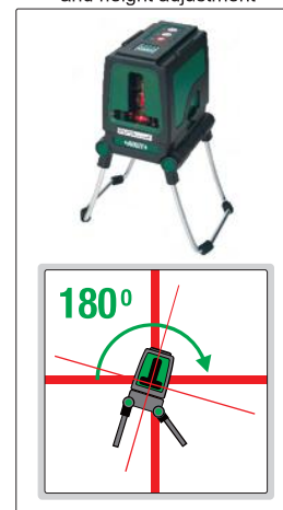
folding legs for angle and height adjustment
